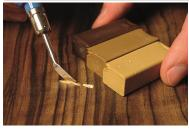
A hard and durable wax filler, designed for repairs to areas subject to severe use. Ideal for repairing edge damage as well as filling holes and scratches of more significant damage. Applied using our range of battery, gas or electric heating irons.
